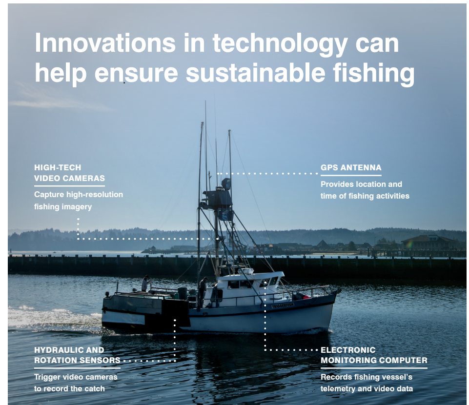
Sample of “making the invisible visible” graphic approach, here using callouts knocked out to white on full-color photography.
